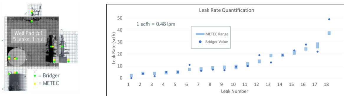
**Figure 1. Left: Round 1 localization results for Well Pad #1 showing actual locations (yellow) and Bridger measured locations (green). Right: Round 1 quantification results showing METEC emission uncertainty range (light blue bars) and Bridger emission measurements (dark blue dots) for a null and 17 leaks.**
