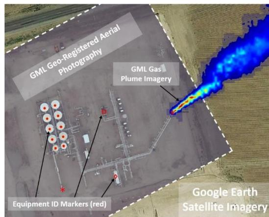
Figure 1. Example of Gas Mapping LiDAR data that is used by operators to efficiently identify and remediate emissions.
